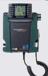
A broad-range measuring device allows for use of the test instrument in all alternating and 3-phase electrical systems with voltages from 65 to 500 V and frequencies of 15.4 to 420 Hz.
