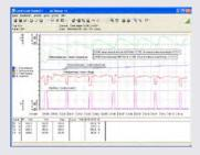
Measured values are queried from the multimeters by METRAwin 10, are managed at PC and can be displayed as Yt or XY graphs (up to 6 channels), or in tabular form (up to 10 channels)
