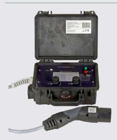
The test instrument is connected to the charging station, in order to document the communication between the charging station and the test instrument. If the charging process doesn't start, the source of error can be quickly pinpointed.
