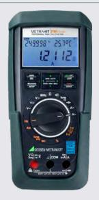
Handheld Digital Multimeter with TRMS Measurement with 100 kHz Bandwidth including amongst others Measuring Functions: V AC TRMS, V AC+DC TRMS, V DC, A AC TRMS, A AC+DC TRMS, A DC dB, Hz(V), Hz(A),  $\Omega$ , V, °C / °F (TC/RTD)
