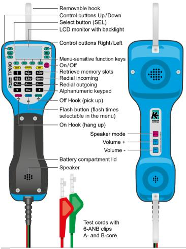
The TP09D is a rugged and waterproof analogue test phone with a back-lit graphic display, protected keyboard, menu-driven operation and caller ID (CLIP), message waiting indicator (MWI), DTMF grabbing, line voltage and current, high-impedance monitor, overvoltage and undervoltage lockout, data security through high-impedance monitor, open listening for monitor and telephony and calling
