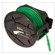
50 m measurement cable coiled onto a plastic drum. Connection to the inside end of the cable is made possible with two sockets integrated into the drum. The other end is equipped with a banana plug.
