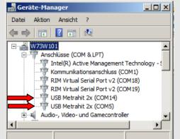
By driver installation an individual virtual COM port is assigned to each adapter. In the Device Manager of Windows, you can verify the success of the installation and identify the assigned COM port number:
