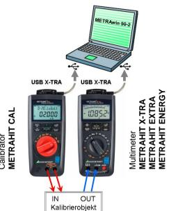
► Each Calibrator and Multimeter is connected via adapter USB X-TRA with a USB port of the PC. <u>Before</u> you connect the adapter to the PC, the driver "GMC Driver Control" must be installed (available on CD or download from website <a href="http://www.gossenmetrawatt.com/english/produkte/drivercontrol.htm">http://www.gossenmetrawatt.com/english/produkte/drivercontrol.htm</a>)
