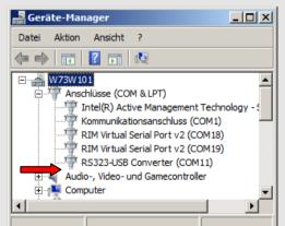
For these converters a driver has to be installed. By driver installation an individual virtual COM port is assigned to each adapter. In the Device Manager of Windows, you can verify the success of the installation and identify the assigned COM port number:
