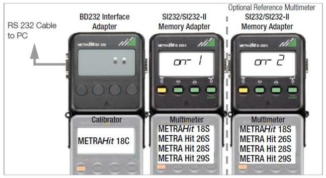
▶ Mount the devices as shown in the illustration and secure the mechanical connections (adapter, cable) using the fixing screws. The connection of a second multimeter with Memory Adapter as a reference multimeter for the measurement of calibration signals, which are not generated by the calibrator (in the TEST program function) is optional.
