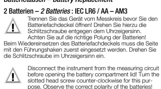
Disconnect the instrument from the measuring circuit before opening the battery compartment lid! Turn the slotted head screw counter-clockwise for this purpose. Observe the correct polarity of the batteries!
