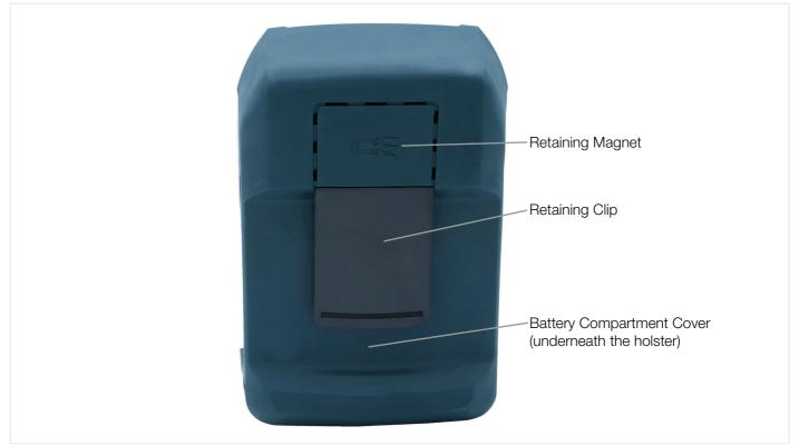
Figure 4: Back of Instrument
