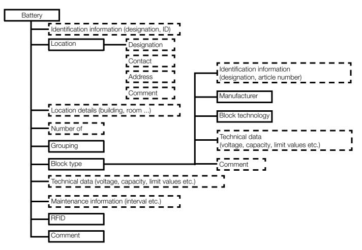
Figure 6: Database Structure – Entries (\_\_\_\_\_) and Storable Information (-----)
