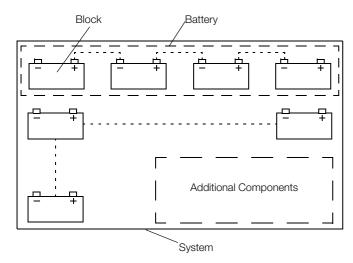
Figure 2: Example – Blocks and Battery within a System
