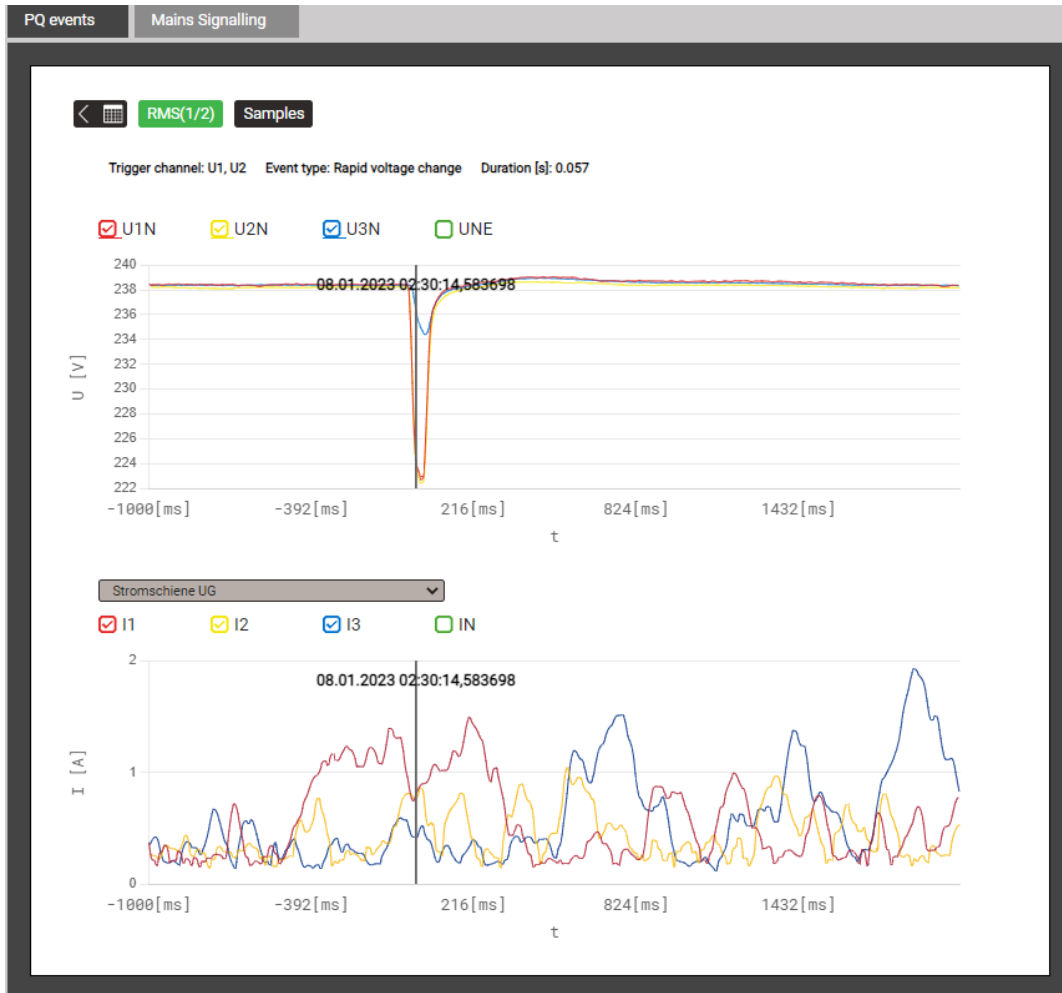
Graphical display of a PQ event (half cycle values), Current module may be selected
