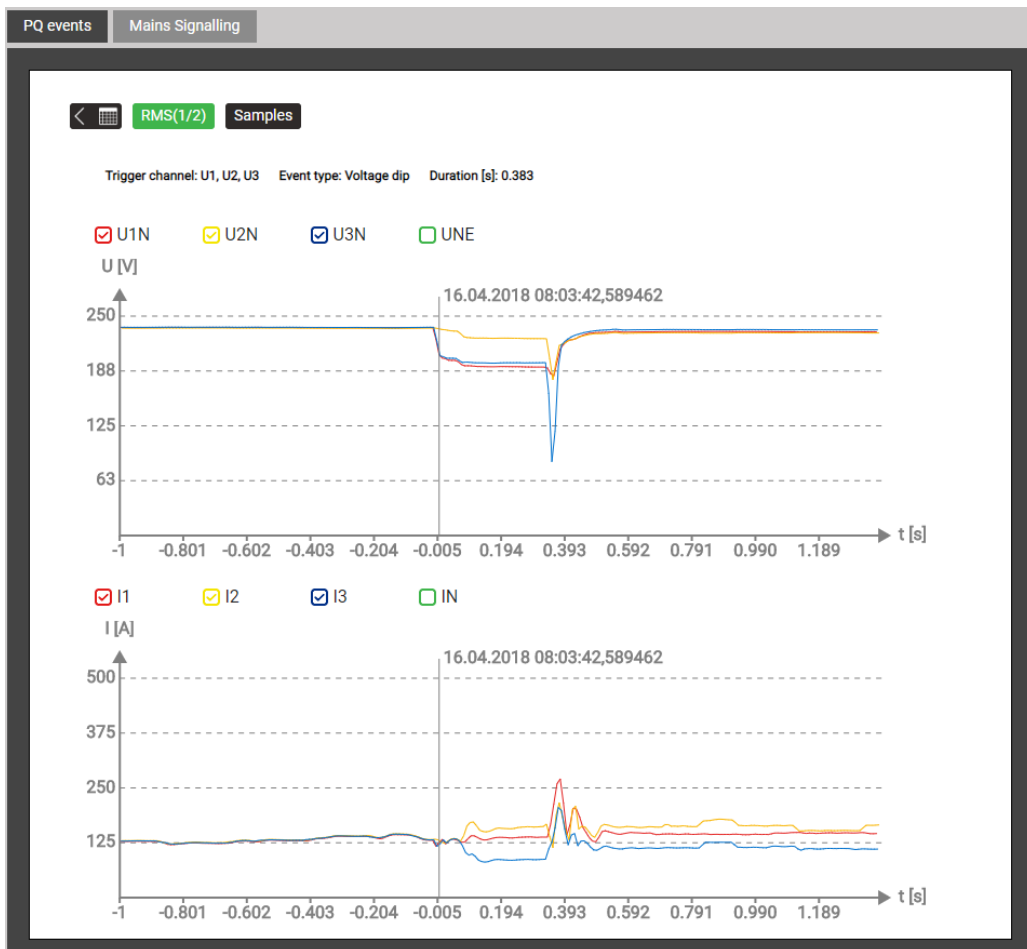
Graphical display of a PQ event (RMS 1/2)
