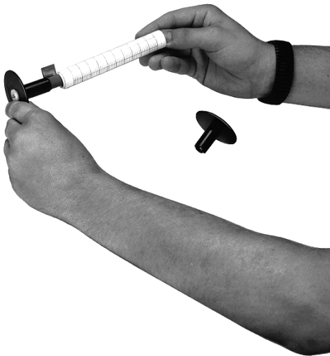
Figure 12 Removing the recording chart from the take-up roll
