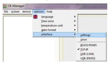
Select "settings" under options | interface. The interface type has to be set to "TCP-IP".
