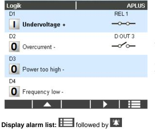
To each alarm a state text for the active and the inactive state can be assigned. The alarm list contains, depending on the present state, either the text for the active or the inactive alarm.
