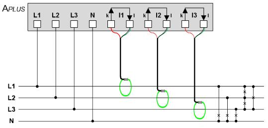
When connecting the coils you must follow the safety notices given in the operating instructions of the Rogowski coil. The current direction shown on the coils must match the real current direction and has to be the same for all phases.
