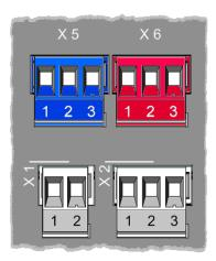
The relay X2 is part of the basic unit and therefore always available. The relays X5 and X6 are provided for device versions with I/O extension PCB only.
