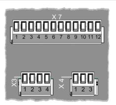
The plug-in terminal X7 is available for device versions with I/O extension PCB only.
