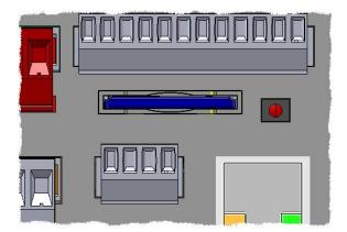
The red LED of the key located next to the SD card signalizes that the logger is active. During writing to the card the LED becomes dark for a short time.
