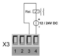
Technical dataRated current50 mA (60 mA max.)Switching frequency (S0)  $\leq 20 \text{ Hz}$ Leakage current0,01 mAVoltage drop< 3 VLoad capacity $400 \Omega \dots 1 \text{ M}\Omega$
