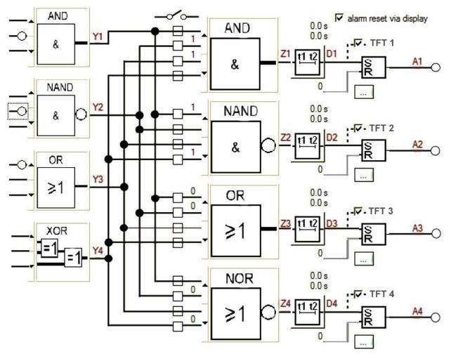
The evaluation of the logic module is performed from top to bottom and from left to right:
