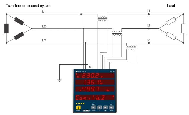
Because in case of a fault the voltage triangle formed by the three phases does not change the voltage and current measurements as well as the system power values will be still measured and displayed correctly. Also the meters carry on to work as expected.
